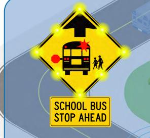
The LEDs begin flashing when the bus passes the sign, and turn off after a preset phase.
