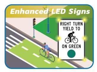
LaneLight LED Bike Signs provide cyclists and motorists with clear, high-visibility messaging to enhance safety and compliance on shared roadways. These signs can be activated by approaching cyclists, ensuring they receive timely alerts about crossings, turns, or potential hazards ahead.
